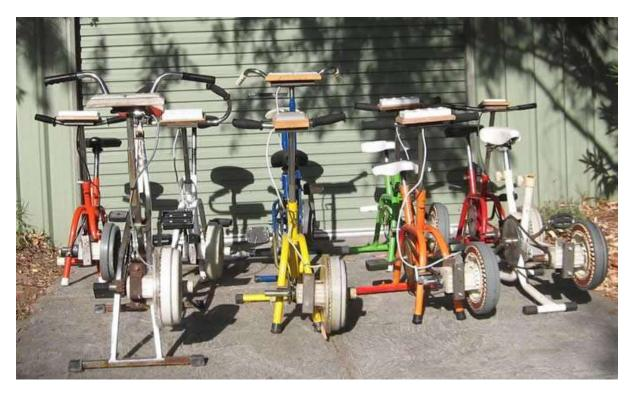
Exercise bike electricity generators capable of running most household appliances. For example the bikes will power (simply plug in), smoothie makers, drills, orbital sanders, lights (LED, compact fluoro, incandescent, halogen), flat screen TVs, computers and laptops and games.
